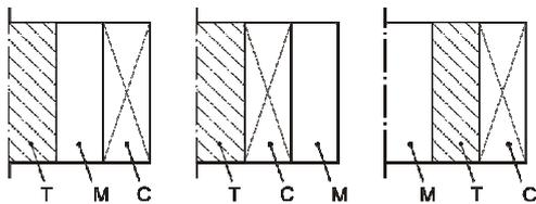
Fig. 3. Sensible configuration of Terfenol rod (T), field coil (C) and permanent magnet (M) (pole shoes not shown)
