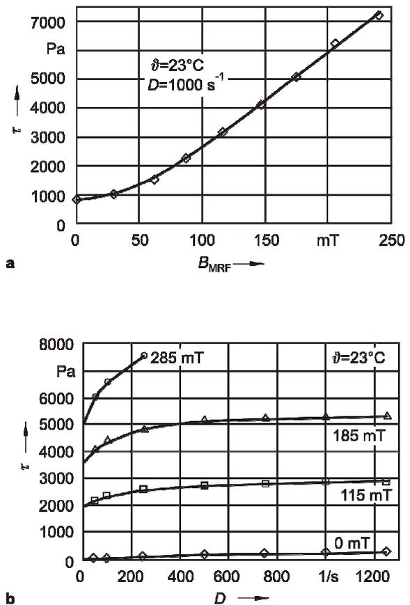
Fig. 6. Characteristics of MR fluid DEA 252: (a) shear stress  $\tau$  as a function of the flux density  $B_{\text{MRF}}$  in the MR fluid; (b) shear stress  $\tau$  as a function of the shear rate  $D$  with  $B_{\text{MRF}}$  as a parameter [10]
