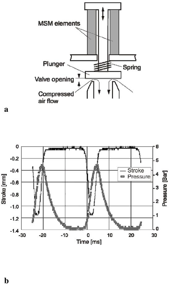
Fig. 12. Principle of a proportional MSM valve: (a) basic structure, (b) pressure and stroke of the valve as a function of time [17]
