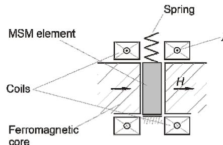
Fig. 11. Basic structure of a linear MSM actuator
