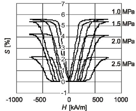
Fig. 10. Magnetic field induced strain  $S$  vs. magnetic field  $H$  of a NiMnGa MSM material
