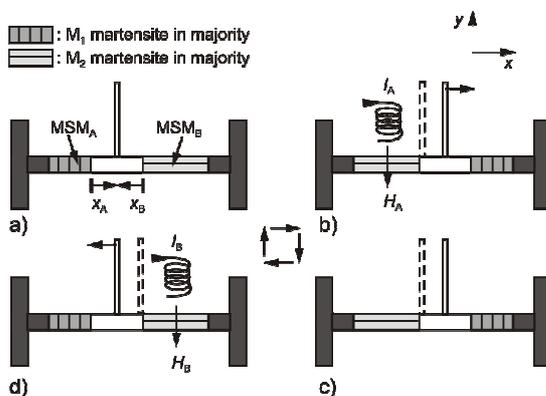
Fig. 13. Principle of a multistable MSM actuator [18]
