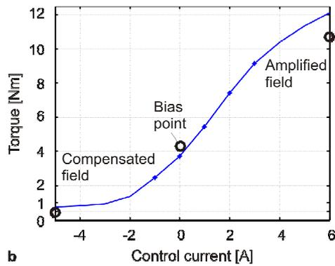
Fig. 9. Vehicle door assistant: (a) basic structure (with amplified field), (b) operating characteristic [14]
