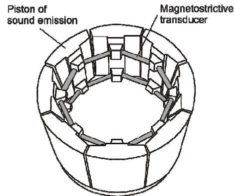
Fig. 4. Basic structure of an underwater sonar system (according to [5])
